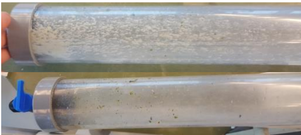
Figure 22 Mold and grease deposits on the collection tube after three weeks of absence.
