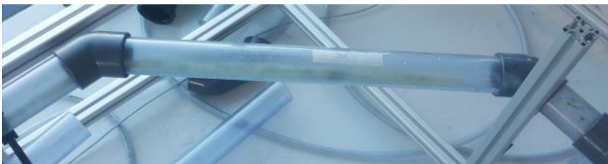
Figure 18 Residual ground food waste in the pipe in the least favourable configuration.
