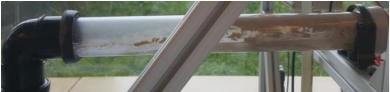
Figure 21 Wall pipe after grinding 250 gr of fat. A flow obstruction occurred.
