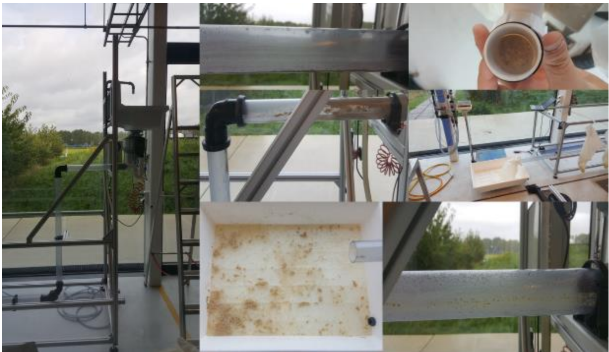
Figure 5. Experimental setup. A typical configuration of a kitchen sink and sewer water pipelines below the sink. The laboratory setup includes a collector at the end of the pipe and sample of residue, which may accumulate in the pipeline.
