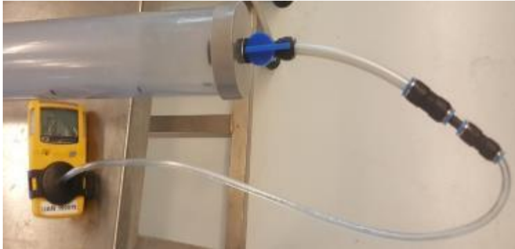
Figure 23 Gas measurements in the sealed horizontal pipe after 3 weeks.
