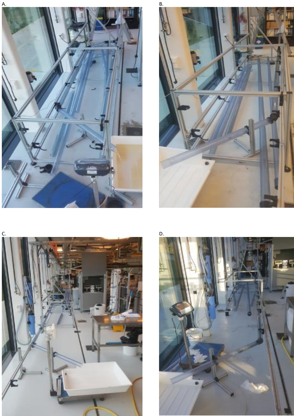
Figure 8 Different lay-out of the pipe configurations. A. 5 meter, 3 bends B. 5 meter, 1 bend C. 8 m, 3 bends D. 8 m, 1 bend
